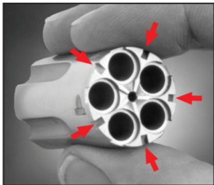
***Hammer safety slots in between cartridge chambers***
