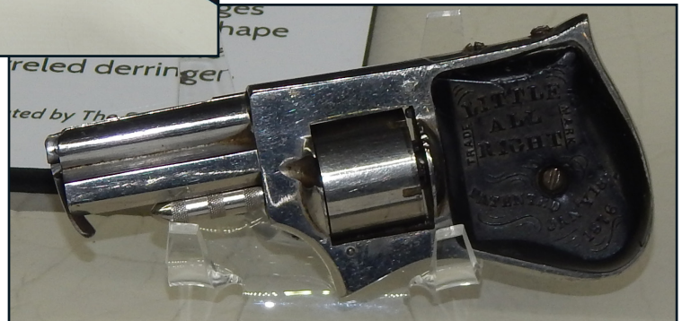
All Right Firearms Co. Little All Right Palm Pistol in .22 Rimfire, circa 1876. Plaque reads: "This diminutive palm pistol requires you to wrap your hand around the entire gun - including the cylinder - in order to engage the folding double-action only trigger mounted on the top of the frame."
