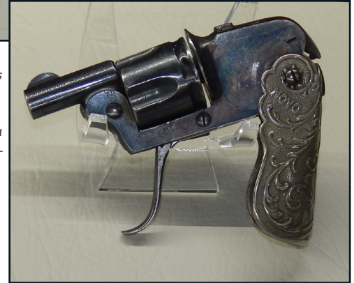
Le Novo Hammerless Folding Trigger Double-Action Revolver in .25 Centerfire, circa 1900 The plaque reads: "Diminutive in size, the Le Novo revolver had a trigger and grip that both folded into the gun, making it incredibly concealable and virtually unde- tectable in your pocket."
