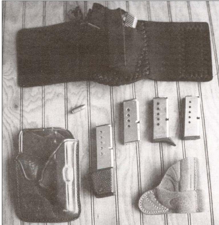
At the top is the Desantis ankle holster. The bottom left shows the Alessi pocket holster with the Ahern holster on the right. The magazines from left to right are the 10-shot extended mag followed by the original 6-shot mag without the extension. The next two are both 6-shot mags, the first with a finger extension and the second with just a black floor plate.
