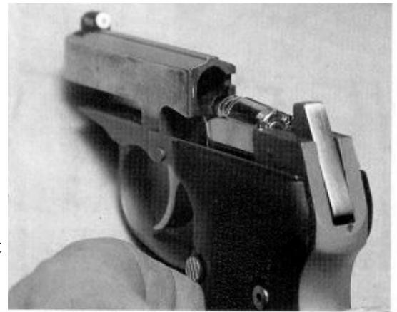
The bottleneck case shape of the .32 NAA combines with the North American Arms pistol's almost straight feed into the barrel to ensure very reliable feeding.
