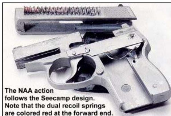
The NAA action follows the Seecamp design. Note that the dual recoil springs are colored red at the forward end.
