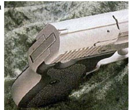
The spurless hammer of this double-action-only design fits flush with the rear of the slide.
