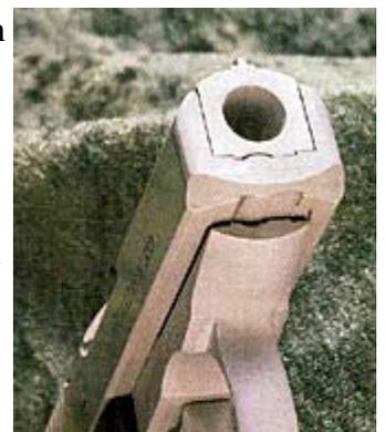
The barrel of this pistol is integral with the frame; the forward portion of the slide leaves the top of the barrel exposed.
